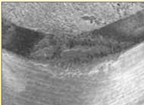
Good GG25 (0.05 S) 62 km sliding distance @ 1500 m/min
